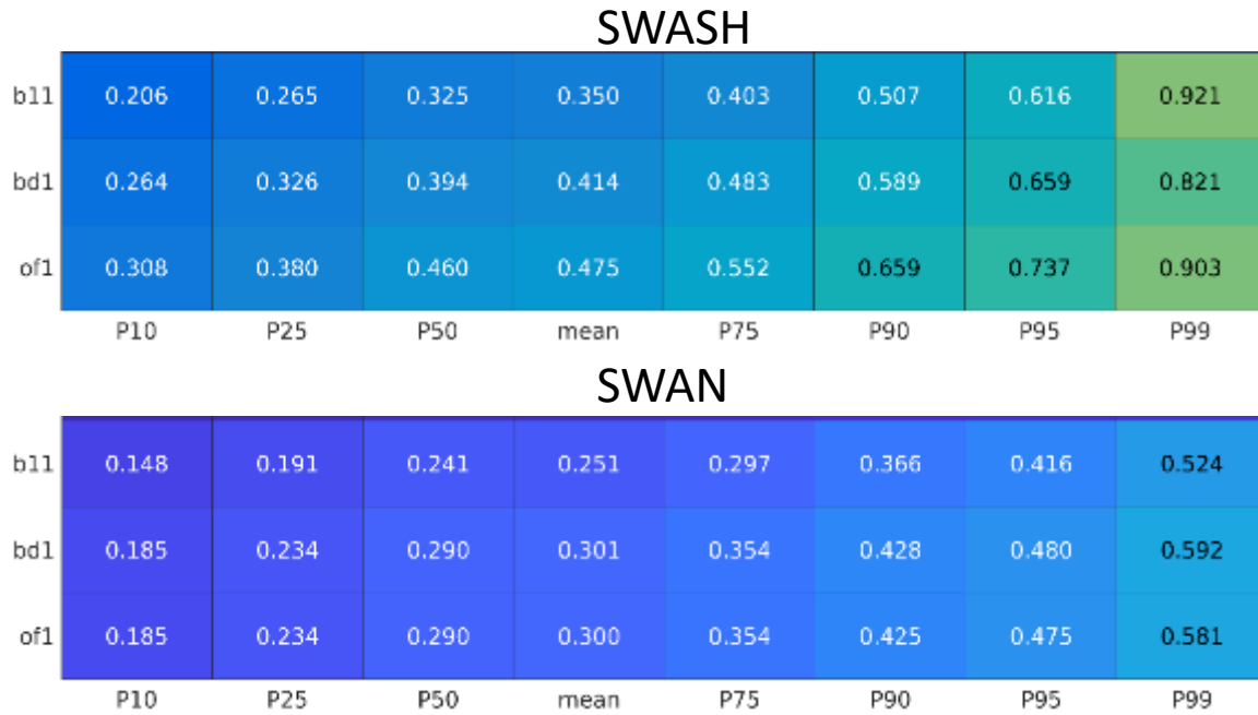
Figure 6. Comparison of significant wave height statistics derived from 10-year timeseries predicted at sites of1, bd1, b11, outside of the port (see Figure 3, bottom panels) by SWAN and SWASH.
